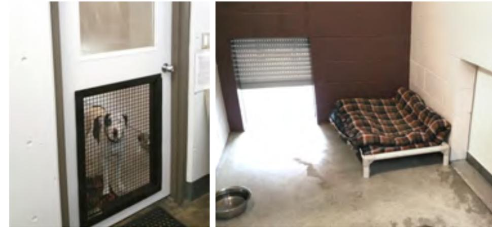
**CLOCKWISE FROM TOP LEFT** A dog awaits adoption in a custom-designed kennel. The kennel door has a glass upper portion, allowing viewing and light entry. The lower portion is an open grate, allowing interaction, reward-based training at the cage front, and air flow. The lower portion can be covered with a sliding panel.
