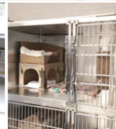
A custom-designed double-compartment dog kennel with a guillotine door allowing outdoor access. The guillotine door is off-centre, providing a hiding space behind the wall. A second door on the side wall leads to a similar kennel and can be left open, creating a double kennel for bonded pairs or dogs requiring more space. Concrete block walls and sealed concrete floors are easy to clean.
